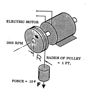
In the example below, the electric motor lifts a 10 pound weight by winding a rope around a 2 foot diameter drum. If the motor is rotating at 1800 RPM, the horsepower produced is 3.4 HP, (see calculations below).
