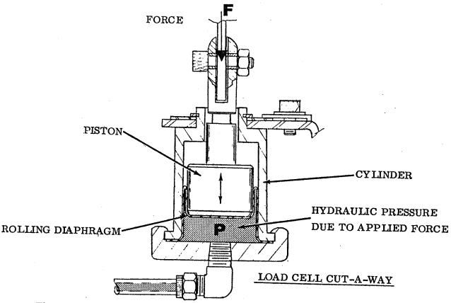
The load cell consists of a piston and cylinder sealed by a rolling diaphragm. This special diaphragm has very low friction and hysterysis as the piston moves. When a force is exerted on the piston by the absorption unit, a hydraulic pressure is generated in the load cell and transmitted to the pressure gage.
