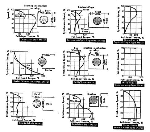
On the motors with centrifugal phase switching, the switch generally is activated at 80% to 90% of the maximum motor speed. An 1800 RPM motor will switch phases when loaded down to 1400 to 1600 RPM. On some motors, you can continue to test the motor on past the phase switching point, but others will stall out due to the shape of their torque curves.
