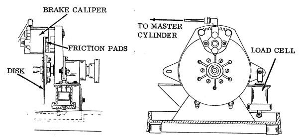
The hydraulic brake master-cylinder contains a by-pass system which automatically compensates for pad wear or loss of hydraulic fluid. The by-pass can be actuated by turning the load control knob all the way out (counter-clockwise). If the brake does not develop full torque when the load control knob is turned all the way in, back the knob all the way out to re-fill the system thru the by-pass and then re-actuate the load system.
